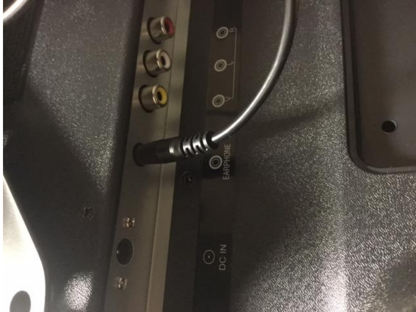
Image 3 - Shows the connection from the Soundbar into the TV for sound. The correct lead has two 'silver male' ends.
