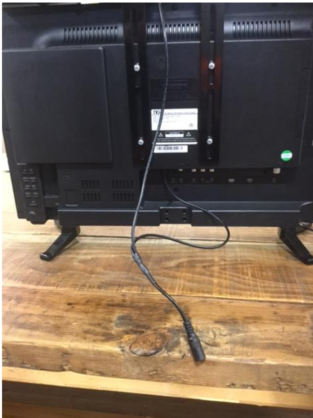
Image 3 - Shows the connection from the Soundbar into the TV for sound. The correct lead has two 'silver male' ends.
