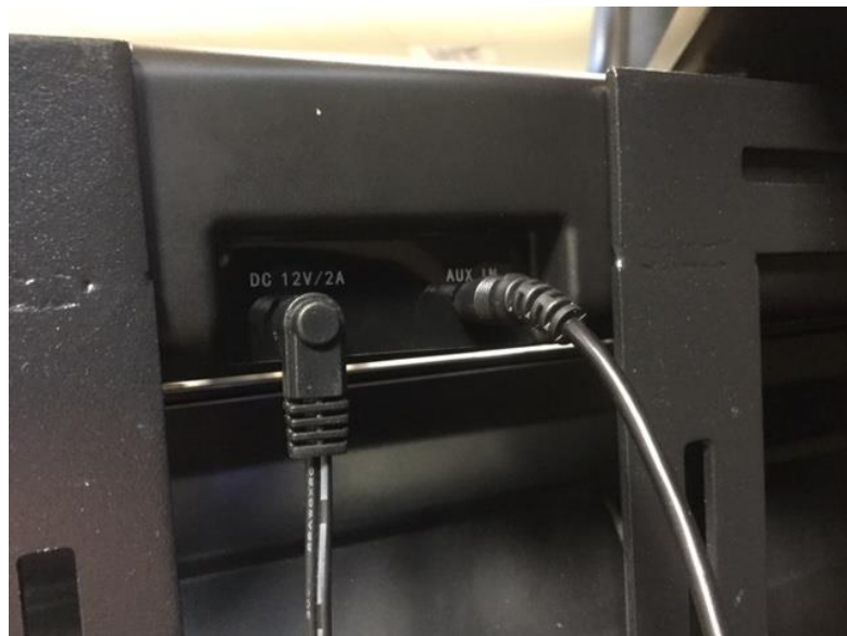
Image 2 - Shows the connection into the rear of the soundbar. Make sure all connections are firm.
